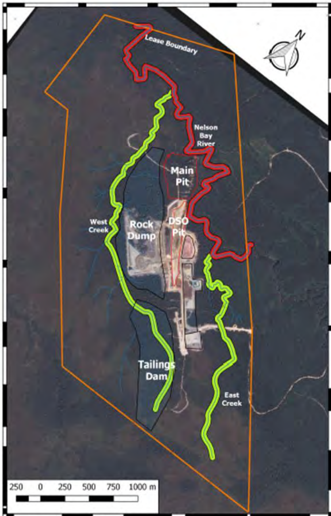
Shree Minerals Nelson Bay River site layout - approximate only, subject to detail survey and design. 30m buffer zones shown for East and West Creeks and Nelson Bay River. Map rotated 38 degrees relative to MGA94 Z55. Scale 1:20,000.
